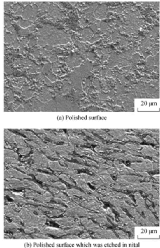
Fig. 4 Microstructure of samples of 30% $\text{Cr}_2\text{AlC}$ /70%Fe sintered at 1 300 °C under 30 MPa for 30 min
