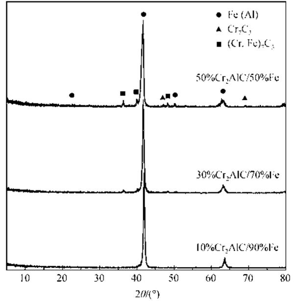
Fig. 3 XRD patterns of samples of  $\text{Cr}_2\text{AlC}$ -Fe mixtures with different  $\text{Cr}_2\text{AlC}$  contents after sintered at 1 300 for 30 min
