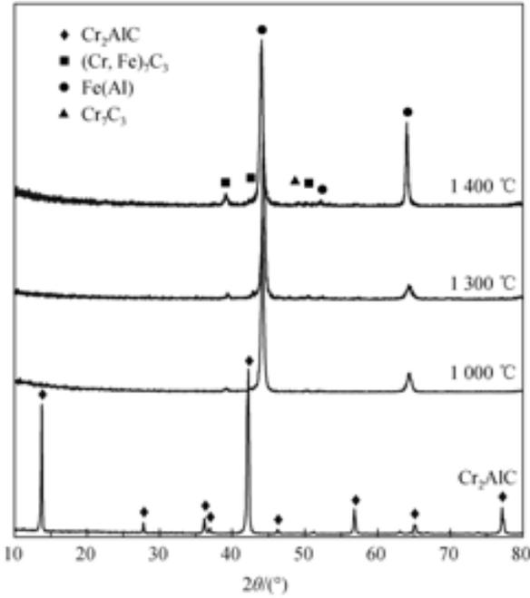
Fig. 2 XRD patterns of  $\text{Cr}_2\text{AlC}$  powders and samples of 30% $\text{Cr}_2\text{AlC}$ /70%Fe composites sintered at 1 000 to 1 400
