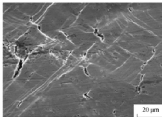
Fig. 7 Typical bending site specimen photograph of 30% $\text{Cr}_2\text{AlC}/70\%\text{Fe}$  sample sintered at 1300 for 30 min after bending tests
