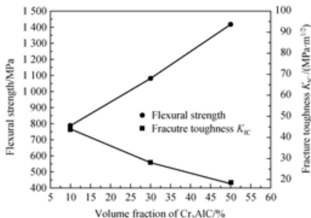
Fig. 6 Relationship between the flexural strength, fracture toughness and the volume content of  $\text{Cr}_2\text{AlC}$  for  $\text{Cr}_2\text{AlC-Fe}$  composites sintered at 1300 for 30 min
