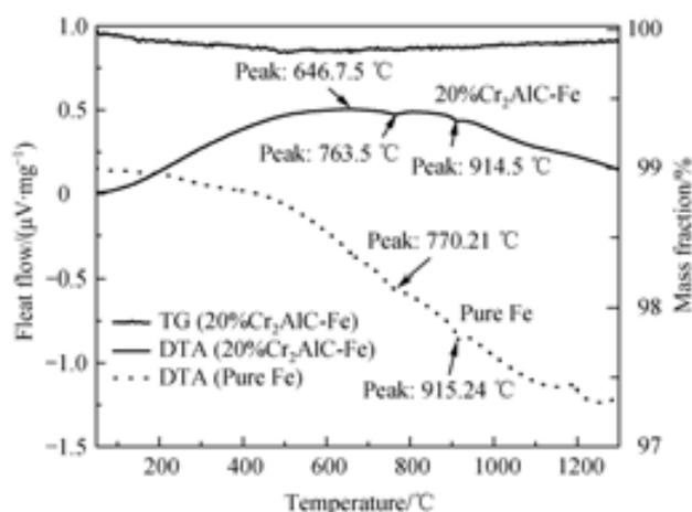
Fig. 1 TG–DTA curves for 30%  $\text{Cr}_2\text{AlC}/70\%\text{Fe}$  and DTA curves for pure Fe powder in argon atmosphere
