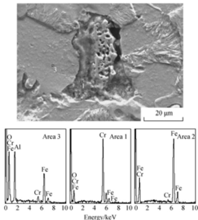
Fig. 5 EDX of samples of 30% $\text{Cr}_2\text{AlC}/70\%\text{Fe}$  sintered at 1300 under 30 MPa for 30 min
